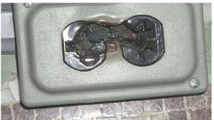
To the left is a burned and melted outlet found in a Congressional facility by the Office of Compliance on a fire safety inspection. This outlet is the result of electrical current overloading and an obvious safety hazard.
